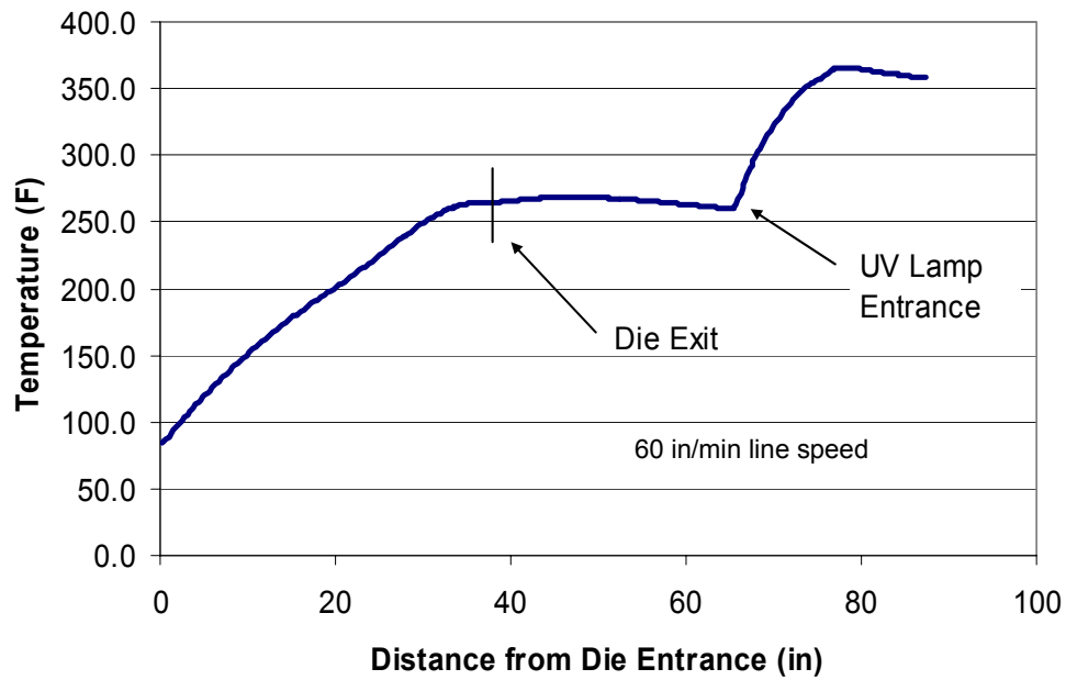
Figure 2. Thermocouple data from the UVPul-OnlineUV experiment showing exotherm from hybrid thermal/photo cure pultrusion using online photocure exposure after the heated pultrusion.
