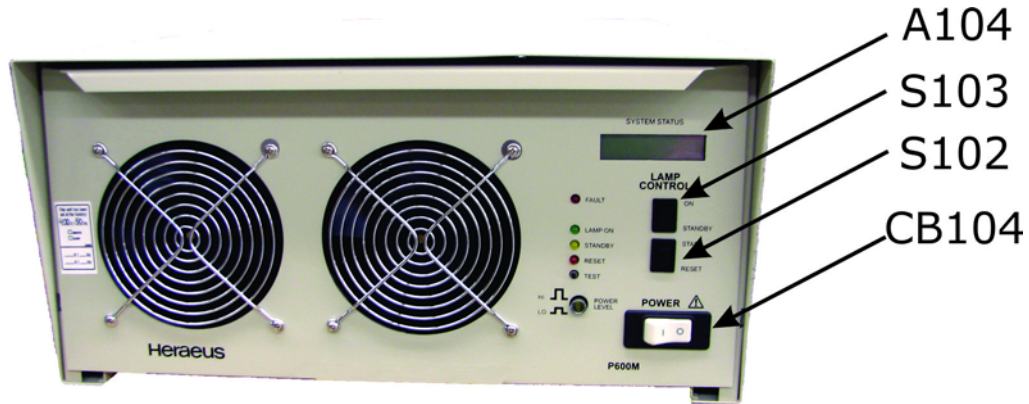
P600M Power Supply Components (Front)
