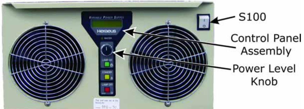
VPS Power Supply Components (Front)
